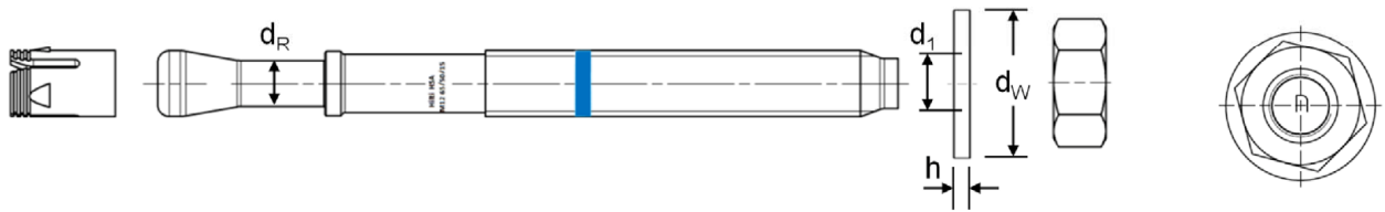
Figure A2: Hilti metal expansion anchor HSA-BW
